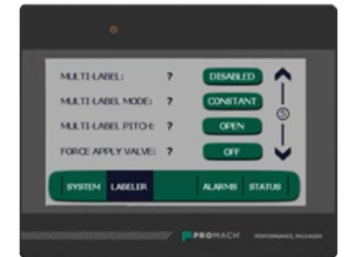
Multi label mode. On-board help for every setting and function by clicking on the "?".
