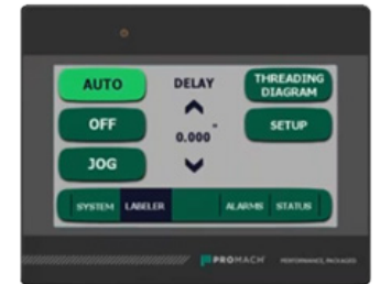
Labeler controls with auto, off, jog, threading diagram, setup, and delay.
