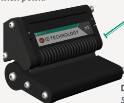
TENSION ROLLER ASSEMBLY Easy to view, centralized nip open lever with magnetic "closed" position. Enclosed nip drive is safer than open nip drive designs, and eliminates a pinch point.
